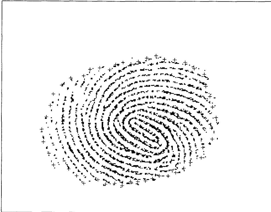
Figure 4-12: An estimate of the overall contact region boundary using the modified wedging method.
