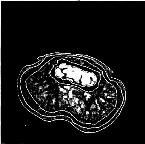
Figure 7.4.9: Fingerpad indented to 1 mm with a 1/8" diameter cylinder.
