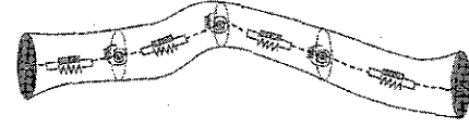
Fig. 8. The catheter was modeled as a set of particles that were uniformly distributed along its centerline. In this model, each particle, moving under the influence of internal and external forces, has a mass and is connected to its neighbors with linear and torsional springs and a damping element. The graphical deformations of the catheter were simulated using a spline-based model coupled with the particle-based model.
