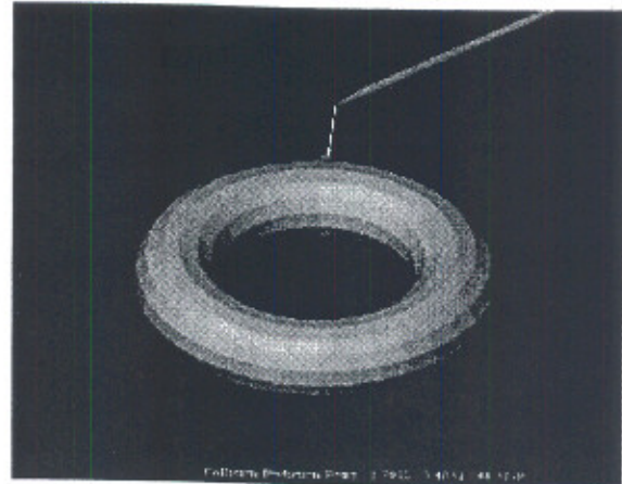
Figure 4. The collision prediction for a 3D object. The small ball on the surface represents the predicted point. The white line is the mean tool path.
